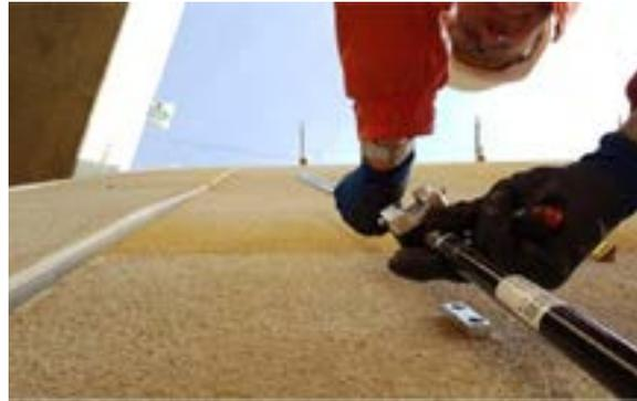
Used vertically in geotechnical applications, FlexiMeasure™ provides a modern carbon fibre in place inclinometer (IPI) solution to measure lateral ground movement in a range of applications. Examples include:
